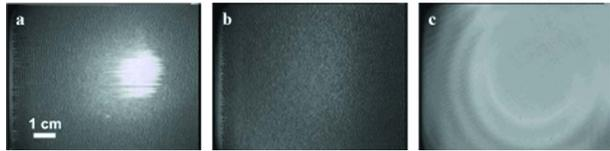
**Fig. 16** CCD camera images of the beam focused by Fresnel lens on Si substrate (a), passing through plain ChG film on Si substrate (b) and direct laser beam (c). The scale bar in (a) is applicable to both (b) and (c).
